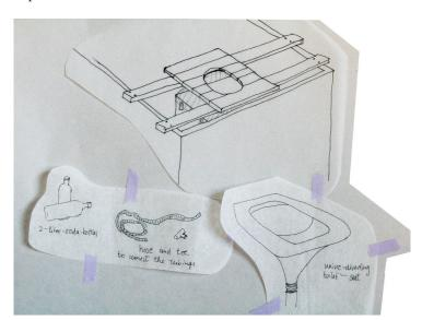
**5** Drill a series of small  $(\frac{1}{4}")$  holes around the top half of the bottle, drill one in the center of the cap. Now drill a hole just large enough to fit the hose, on the sides of each bottle towards the bottom of each bottle.
