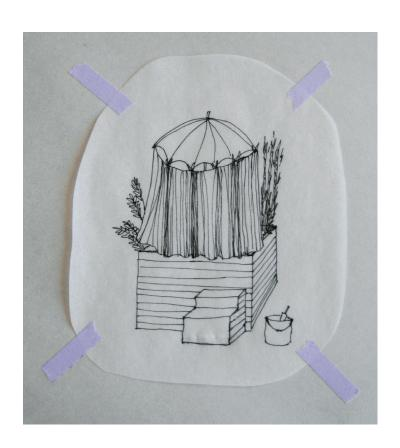
Next, assemble a platform with a hole for the toilet seat. Secure it on the front (long) edge of the planter. Put a cardboard box directly below the toilet seat.
