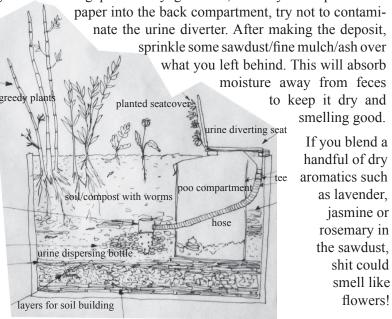
This is how the parts are working together on the magic transformation of HUMAN WASTE into HUMANURE.
